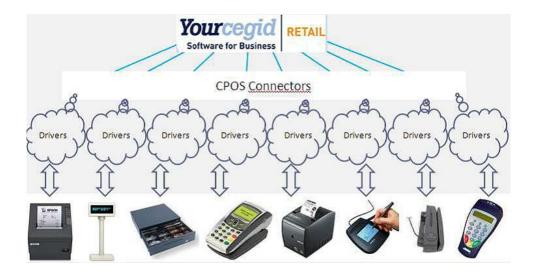
Instead of exchanging directly with each device, the POS terminal communicates with a generic multidevice connector called CPOS.
